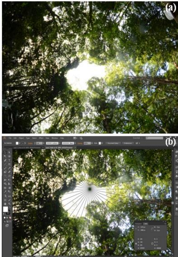
Figure 2. (a) The gap photo taken by fish eye lens camera; and (b) the measurement of length in pixels by Adobe Illustrator CC 2014 computer software program
